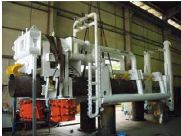
Figure 1. Tiger Shark Jet, mechanical trencher.
